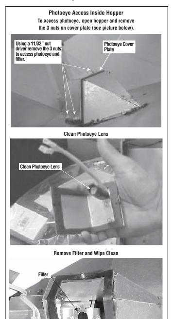
(Minimum frequency of 4 weeks - 6 months) Figure 53 - Clean Photoeye Lens and Filter
